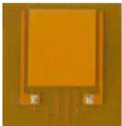
Flexible interdigitated Macro Fibre Composite (MFCs) transducers are proposed for the onset of defect detection. Experimental analysis using MFCs is presented in the TWI paper 'Assessment of Defects in Wind and Tidal Turbine Blades using Guided Waves' submitted to FESI for the upcoming 'ESIA II - Engineering Structural Integrity Assessment' conference on the 24th-25th May 2011 in Manchester.
