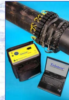
Teletest® is a long-range ultrasonic non-destructive testing technology developed to generate guided waves for detecting metal loss in pipe work when access is difficult. It is a pulse echo system aimed at testing large volumes of material from a single test point.
