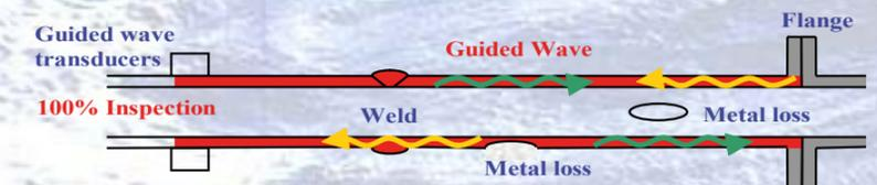
Teletest® is primarily a screening tool with the added feature of focusing the sound energy into a specific region to measure the distribution of the defects for further evaluation using other NDE methods.
