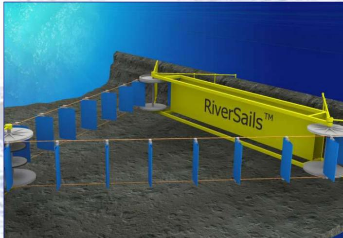
The TidalSails/RiverSails system combines the efficiency of large, low cost energy collector area consisting of multiple wings like sails, with alpine skilift technology.
