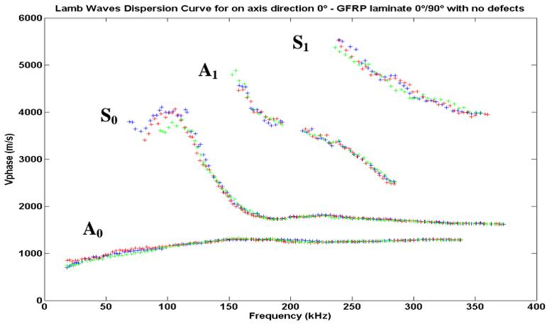
Figure 4: Normalised dispersion curve – bidirectional sample
