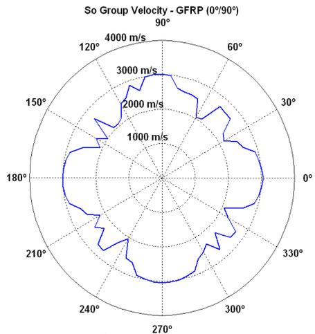
Figure 7:  $S_0$  group velocity in the bidirectional GFRP
