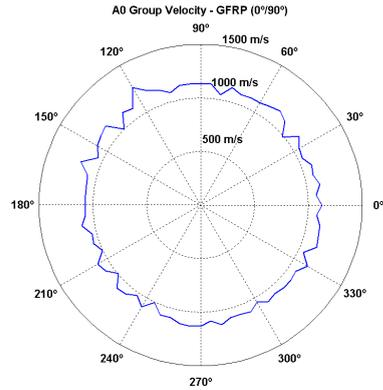
Figure 9: A<sub>0</sub> group velocity in the bidirectional GFRP
