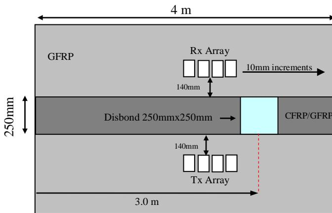
Figure 10: Disbond in spar-cap of blade sample
