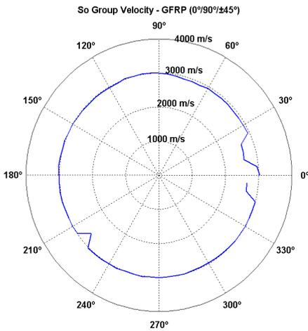
Figure 6:  $S_0$  group velocity in the quasi-isotropic GFRP
