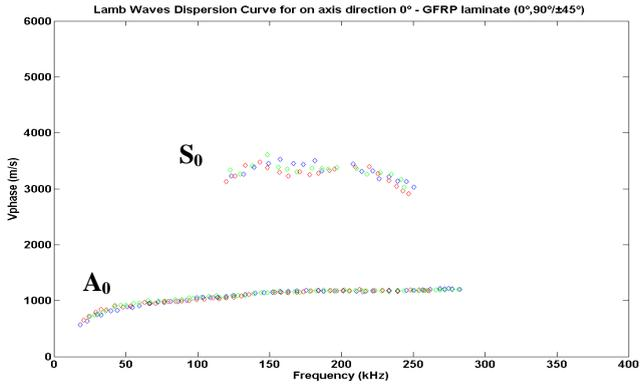
Figure 3: Normalised Dispersion curve - quasi-isotropic sample
