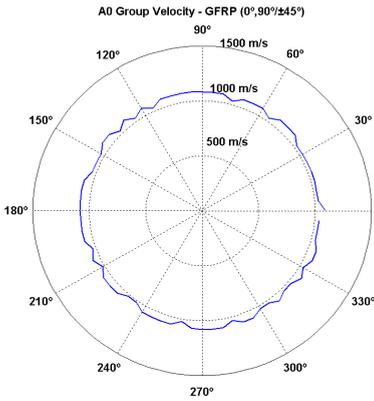
Figure 8: A<sub>0</sub> group velocity in the quasi-isotropic GFRP
